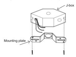
**2.** Connect supply wires to wires on fixture with wire nuts or push wires into Quick Connector. Connect white to white, black to black, and copper wire to copper wire as grounding connection.
