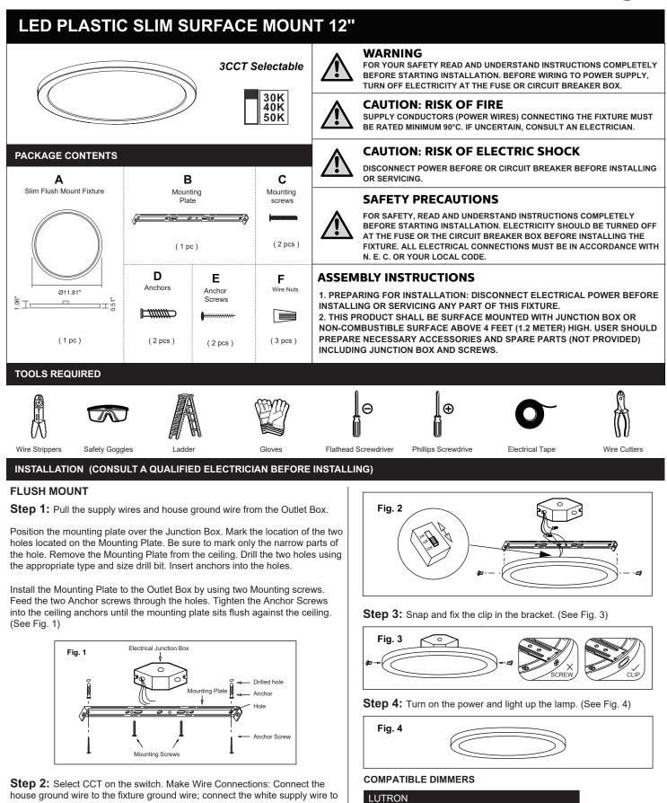
house ground wire to the fixture ground wire, connect the white supply wire to the white fixture wire; connect the black supply wire to the black fixture wire by using the wire connectors. Carefully tuck all wires back into the Junction Box (1). (See Fig. 2)
